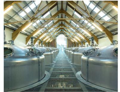
*"All the cooling water, 400,000 litres per hour, comes from the River Spey. The thermal vapour recompression technology [on the spirit condensers] makes this one of the most efficient distilleries in the world."*
